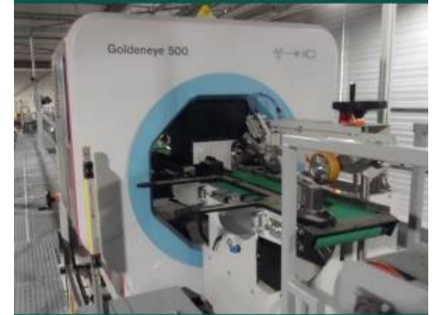
Stacker 2 Scanner: Infrared and x-ray
